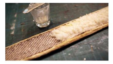
When adding a lining that consists of multiple pieces, it is essential that they overlap downwards, in order to reduce the risk of the blade sliding between layers. When pieces of the lining become loose, and end up buried deep in a scabbard, it is basically ruined (unless it is detachable like e.g. some Iron Age models).
