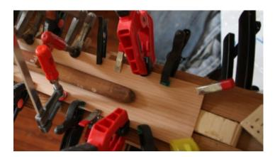
I also pushed a piece of wood under one end to fold up the boards on the side where the scabbard point will be situated later. However, this kind of fine tuning is not actually required at this point.
