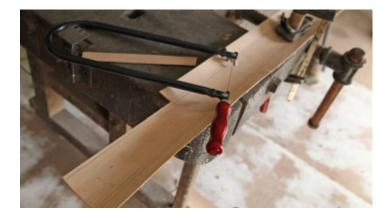
I cut out each shape with a simple coping saw.
