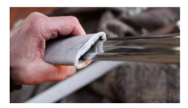
After trimming the excess at the scabbard mouth, and shaping it with some glue (note that the lining should fold over the edges of the mouth!), I can finally insert the blade.
