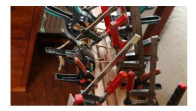
I use additional clamps to join the boards' edges.
