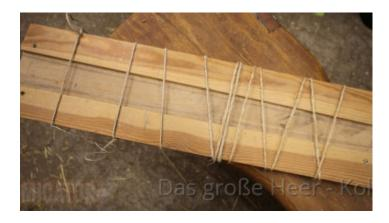
The basic idea is that the two boards are glued together while bent to create a curved scabbard half. To this end, I use a primitive mould consisting of but a wooden board with two wooden laths attached to it. They are not exactly parallel to each other, so that the gap between them is slightly tapering to the lower end. This is the negative form, or matrix.
