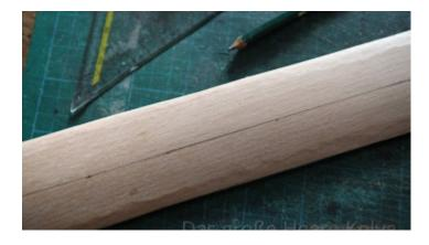
I start by marking a center line on the back of each scabbard.
